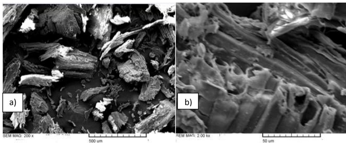
**Figure 2:** SEM micrograph Beech wood sawdust:
