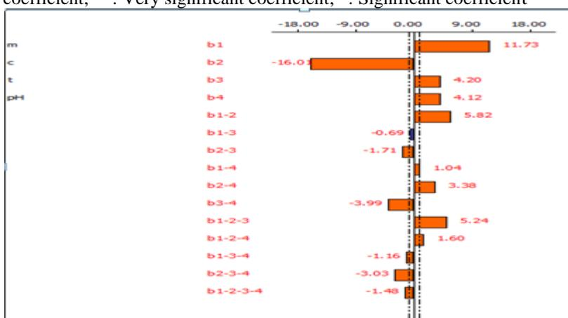
**Figure 13:** The factors effect's graph for methylene blue on beech wood sawdust
